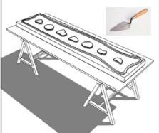
2. Apply a cement based flexible tile adhesive directly to the board. A solid bed of adhesive should be applied around the edges of the board with centre dots at a maximum of 300mm centres. Maximum adhesive dab thickness should not exceed 30mm thick
