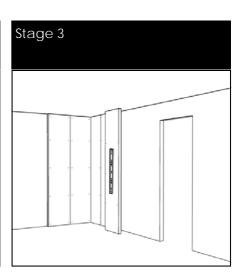
Offer up the board vertically to the wall surface and bed firmly into place.
