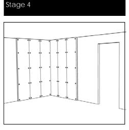
4. Once the adhesive has set approx. 48 hrs, mechanical fasteners/dowels should also be used. Position the fasteners at approx.600mm centres fixed through the centre of the hardened adhesive.
