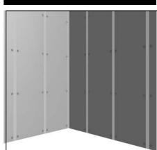
All gaps and joints must be taped prior to tiling with a suitable reinforcement tape.
