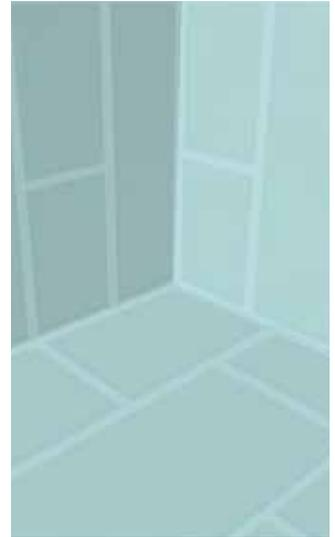
**STAGE 6** Once the Tanking Paste is fully cured, your sealed surfaces are ready to be tiled. The drying/curing time will depend on the porosity of the substrate, thickness of the Tanking Paste applied and the ambient conditions/temperatures. In ideal conditions, tiling can commence approximately 3 hours after the second coat of paste has been applied. Please note – in poor conditions, the drying process can take up to 24 hours.
