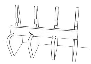
2) Mark the positions of the supporting panels A on strut C1.
