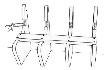
5) Apply BOARD-FIX® to the recessed area for strut C2.
