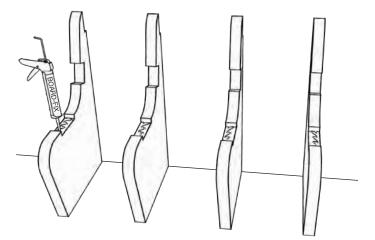
3) Apply BOARD-FIX® to the recessed area for strut C1.
