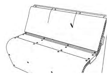
**18)** Fit cover B3 and mark the positions for the middle supporting panels.
