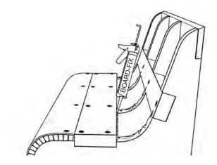
**14)** Apply BOARD-FIX<sup>®</sup> to supporting panels A and to the long side of strut C1.
