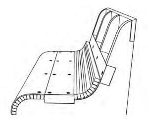
**15)** Prebend cover B2 before gluing on to relieve the tension. Then glue on cover B2 with the slotted side facing upwards.
