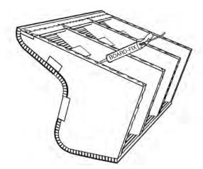
**22)** The bench must be glued to the wall and the floor. To do this, apply BOARD-FIX<sup>®</sup> to the front surfaces of the back and underside.
