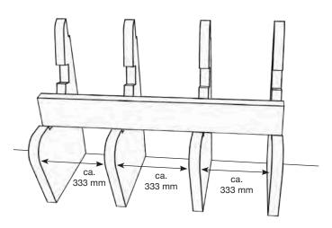
1) Set up supporting panels A an equal distance apart.
