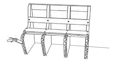
10) Apply BOARD-FIX  $^{\mbox{\tiny B}}$  to supporting panels A and to the long side of strut C1.
