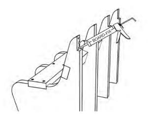
7) Apply BOARD-FIX® to the recessed area for strut C3.
