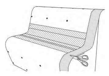
**24)** Tape over cover B2, all butt joints and visible edges with JACKOBOARD<sup>®</sup> self-adhesive glass fibre tape.
