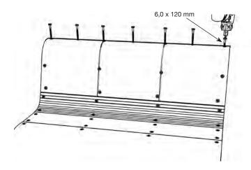
19) Apply BOARD-FIX® to supporting panels A, strut C1
