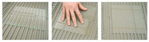
Wettability test: a simple pressure is enough to obtain full-bedding under the tile
