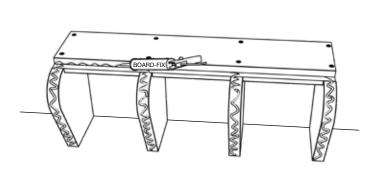
7) Apply BOARD-FIX® to supporting panels A and to the long side of cover B1.
