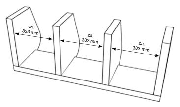
1) Set up supporting panels A the same distance apart on the underside of cover B1...
