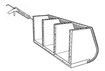
**11)** The bench must be glued to the wall and the floor. To do this, apply BOARD-FIX® to the front surfaces of the back and underside.
